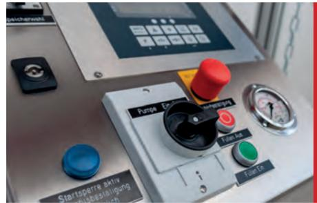
• The filling process is programmed and controlled at the freely placeable and height adjustable control desk of the CFA 5.
