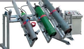
• Testing and swivelling device big cylinder PSG with HTG 500.
