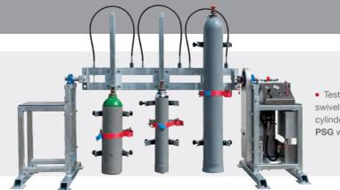
electric motor and roller chain. The tested cylinders are very easily turning them 180 degrees in both directions. The used water can be and used again with the help of the optionally available collecting ta
