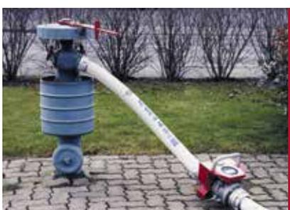
• Flow measurement at pillar hydrant.
