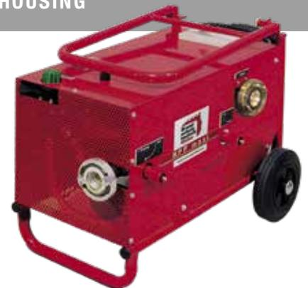
The adjusted pressure can be read at the glycerine-filled manometer. The automatic non-return valve prevents return flow during pressure build-up. Handling is easy: The test object is filled with water via the ball valve at the device. Then the pressure is built up. After the test, a second ball valve decompresses the pressure.
