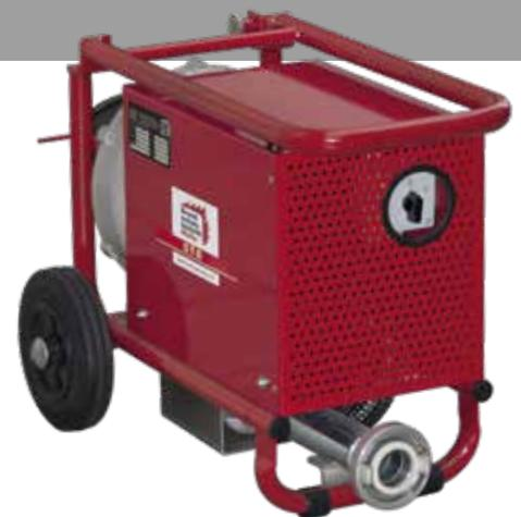
The device is composed of a steel pipe frame with wheels, an electric motor with side channel blower and flanged air heater, an adjustable thermostat and a Storz C coupling connection. Motor, air heater and thermostat are protected by a galvanized sheet steel housing. A 5 m cable and cam switch supply the power.
