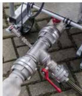
After checking the line for completeness and the valves and other facilities for functional capability, the line must be filled with water completely. The **hydrant testing pump HPP**, flow measurement meter **DMT 600** and riser pipe are connected in the process. The static pressure test can be subsequently performed with the **hydrant testing pump HPP**. The pressure difference at specified rate of flow of 600 L/min is determined following the pressure test.
