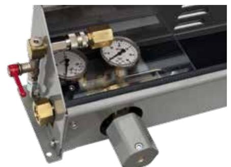
• Manometers for inlet and test pressure.
